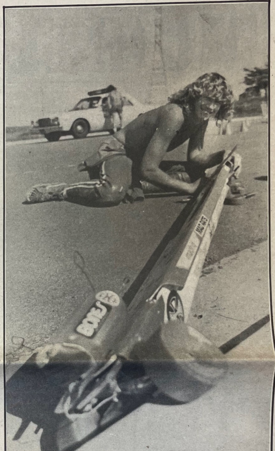
What it takes to go down the hill fast. It weighs 65 pounds, large fast wheels, parachute optional.
